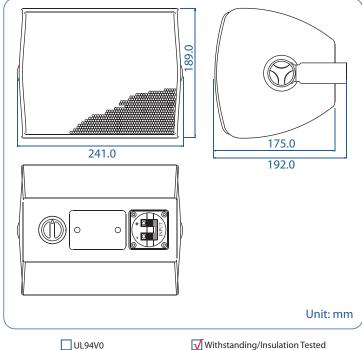
➤ Very high quality 2-way speaker system with 5" polypropylene bass / mid cone & 10-ounce magnet + mylar laminate dome tweeter
